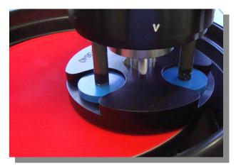
During operation, the individual pistons will extend from the cylinder body to apply pressure to the back of the mounts. Where there is an empty location, the piston stops above the platen surface so it does not make contact.
