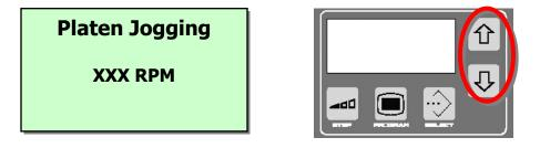
Change the platen RPM using the arrow buttons (circled above) to the right of the display.
