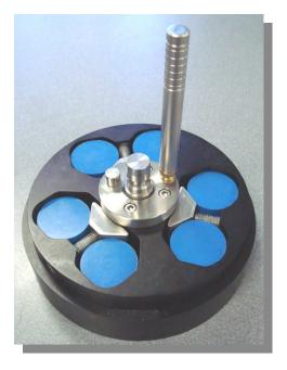
To secure, apply pressure to the backside of the mount/sample and tighten the set-screw (tear-drop shown).
