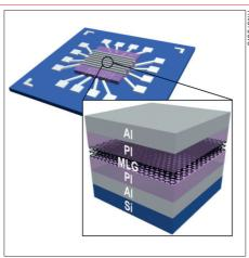
**Smart storage** Multilayer graphene acts as a charge-trapping layer in organic memory devices.
