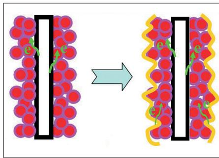
**High-performance coating** Graphene/manganese electrodes dipped into a carbon-nanotube solution.
