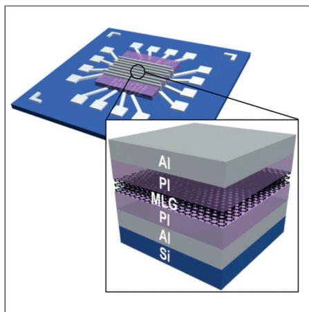
**Smart storage** Multilayer graphene acts as a charge-trapping layer in organic memory devices.
