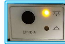
2. Adjust **Bright/Dark Field** selector lever to desired
