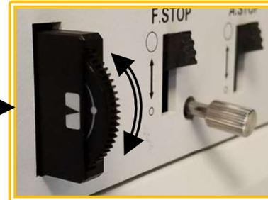
5. Rotate the polarizer to adjust the polarization from
