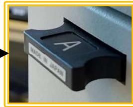
4. Push the **Polarizer Slider** in  $\Rightarrow$
