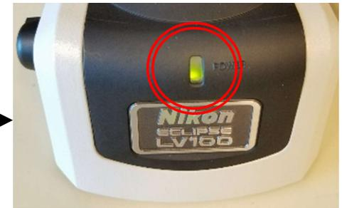
10. If light is missing, turn on **Lamp Power Switch** on back
