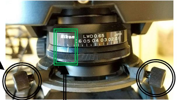
9. Focus on specimen by adjusting the **Coarse/Fine Focus** knobs
