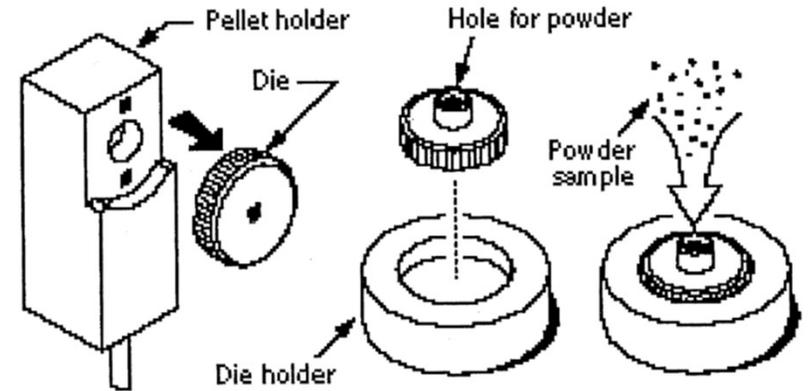
4. Place **Metal Cylinder** over **Die** with the small hole facing up
