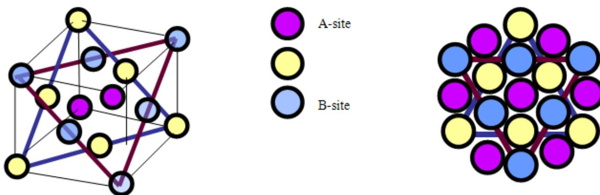
**Fig. 6.2** FCC structure viewed from direction [111];
