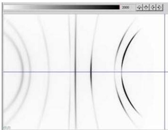
**Fig. 5.11** Diffraction profile of rolled copper plate. Variation of intensity is seen along the Debye-Scherrer diffraction ring, but with certain recognizable regularity.
