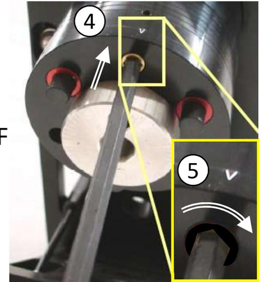
7. Take a  $\frac{5}{32}$  **Allen Wrench** and securely tighten the set-screw
