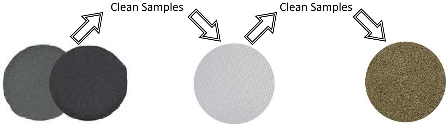
2. Failure to properly clean each **Sample** before next step will transfer **Abrasive Particles** onto subsequent **Grinding Paper** and **Polishing Cloth**
