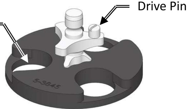
**Sample Loading/Unloading Fixture**
