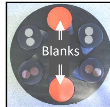
13. Secure the **Sample Mounts** by applying pressure to the backside of the **Sample Mount** and tightening the set-screw using provided **1/8" Allen Wrench**
