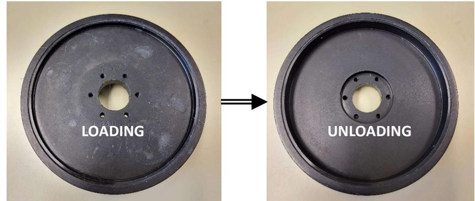
15. Insert the **Sample Holder** onto the **Sample Unloading Fixture** with the **Sample Mounts** facing upward
