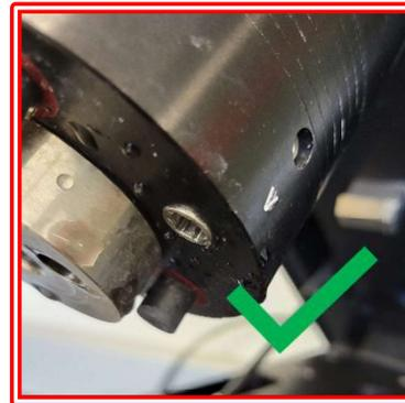
7. Take a  $\frac{5}{32}$  **Allen Wrench** and securely tighten the set-screw
