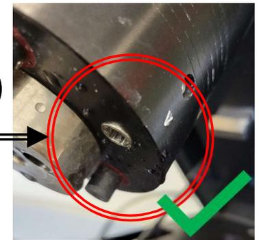
3. If not, locate the “**V**” stamped into the cylinder
