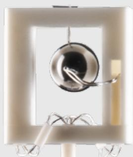
TGA-DTA sensor for hanging samples
