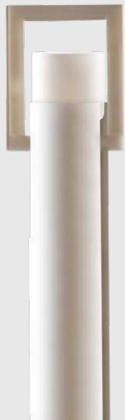
TGA sample carrier for measurements in an immersion bath
