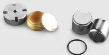
Medium-pressure crucible (right) and high-pressure crucible (left)
