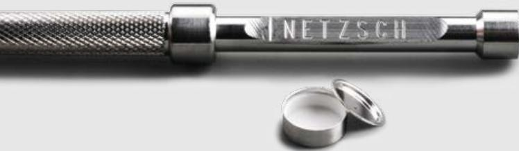
The crucible combination of PtRh/ $\text{Al}_2\text{O}_3$  (order no. 6.225.6-93.2.00) can be used for samples which may react with Pt up to 1700°C. In addition to the  $\text{Al}_2\text{O}_3$  liner, MgO and  $\text{Y}_2\text{O}_3$  liners are also available.
