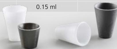
TGA-DTA crucibles for highest temperatures
