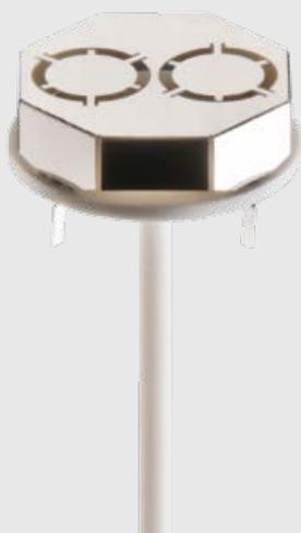
TGA-DTA sample carrier (with protected thermocouples) and slip-on plates for ASC operation
