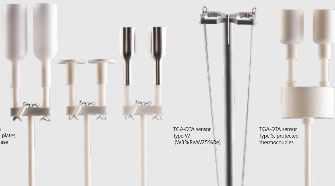
TGA-DTA sensors with different crucibles and plates; for more crucibles, please see TGA
