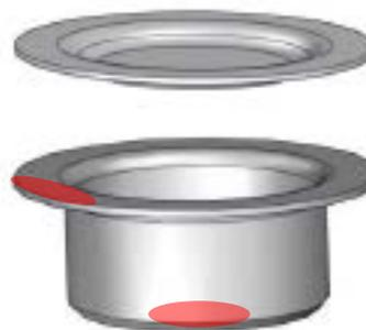
6. Avoid over-filling the crucible in case the sample boils and bubbles over contaminating the DSC sample chamber \$\$\$
