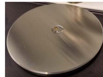
4. To reduce of evaporation place **Volatiles Cover** over sample
