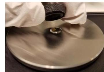
5. Install **Flat Pressure Tip**, move into **Sampling Position**, and lower the **Pressure Tower** until the **Pressure Tower Knob Clicks** and **Freely Rotates** when the maximum pressure is reached
