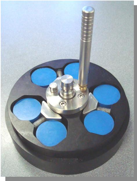
To secure, apply pressure to the backside of the mount/sample and tighten the set-screw (tear-drop shown).
