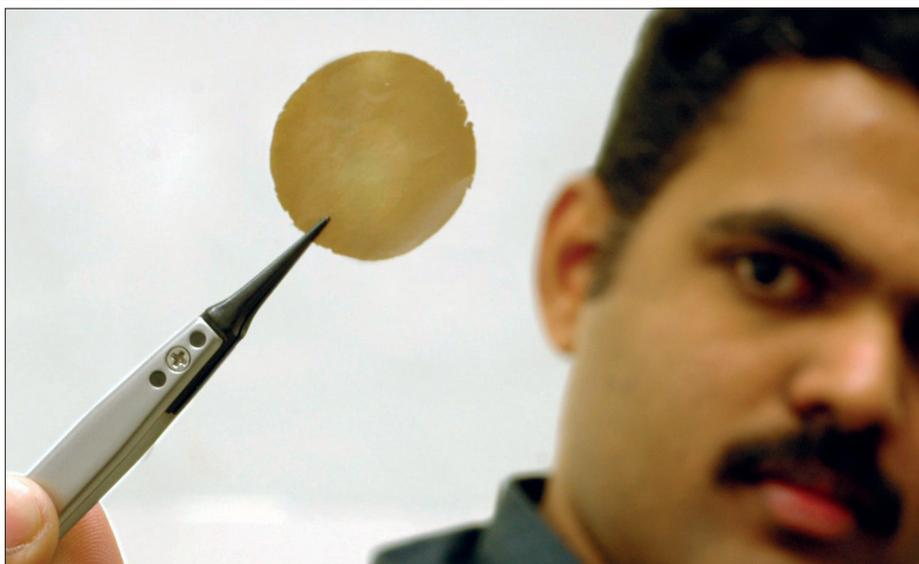
**Magic membranes** Flakes of graphene oxide could be used to separate water from other liquids.
