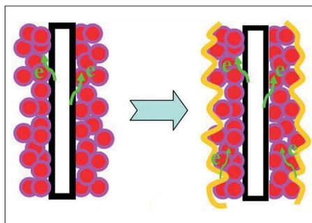
**High-performance coating** Graphene/manganese electrodes dipped into a carbon-nanotube solution.
