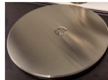
4. For *highly volatile samples*, place *Volatiles Cover* over sample to reduce of evaporation
