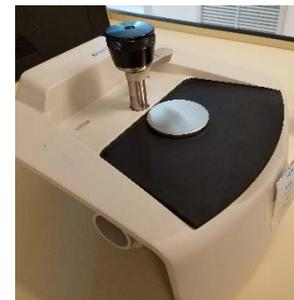
2. Please contact the Lab Manager if you need to use the **Smart Transmission Accessory** for Transmission FT-IR measurements
