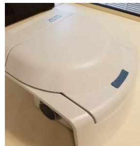
3. The **Smart ATR Accessory** contains mirrored optics that need to be carefully taken care to avoid damage and contamination
