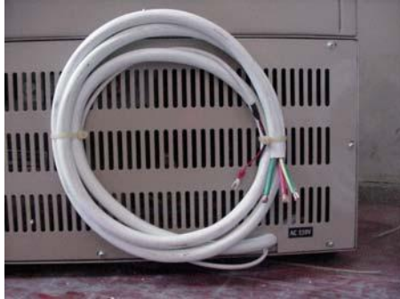
Fig. 23 a: Three power lines from back of furnace
