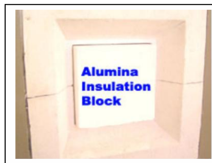
Fig. 24b, Alumina insulation block behind the door of the furnace
