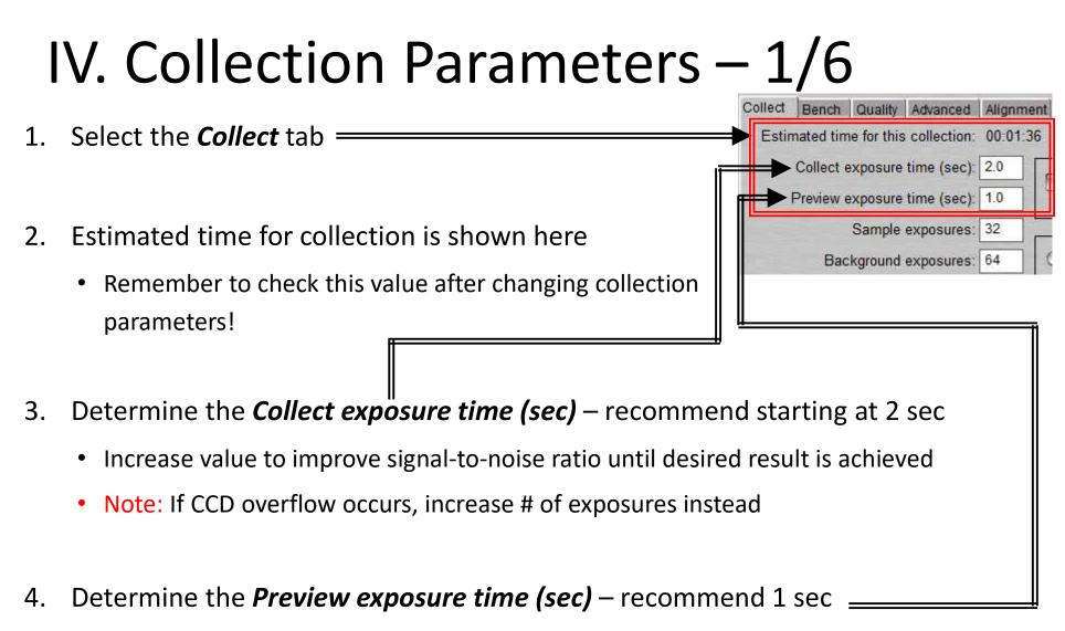
• This value also determines the exposure time for the live display on Bench tab
