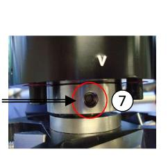
7. Take a 5/32 Allen Wrench and securely tighten the set-screw =
