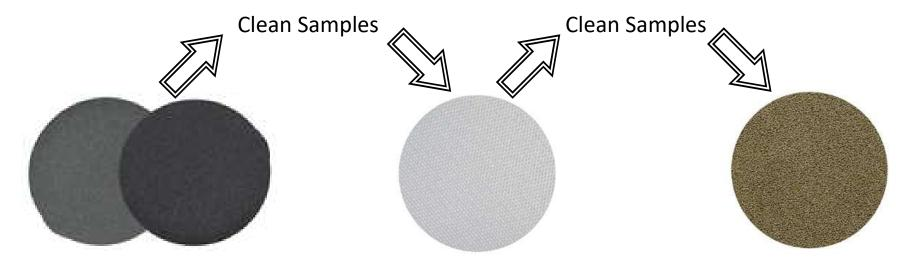
2. Failure to properly clean each *Sample* before next step will transfer *Abrasive Particles* onto subsequent *Grinding Paper* and *Polishing Cloth*
