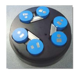
17. Remove the *Samples* from the *Sample Holder* by loosening the set-screw with provided *1/8" Allen Wrench*
