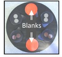
13. Secure the *Sample Mounts* by applying pressure to the backside of the *Sample Mount* and tightening the set-screw using provided *1/8" Allen Wrench*
