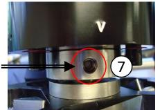
7. Take a 5/32 Allen Wrench and securely tighten the set-screw =
