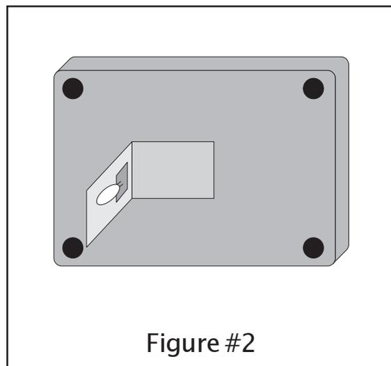
and pulling it from its fixture. When replacing, insert the new lamp into the same fixture. When replacing the lamp, be careful **NOT TO TOUCH THE GLASS ENVELOPE WITH YOUR FINGERS**. Use a tissue or other medium to grasp the lamp. This will prevent oils from your hand from reducing lamp life (see figure #2).
