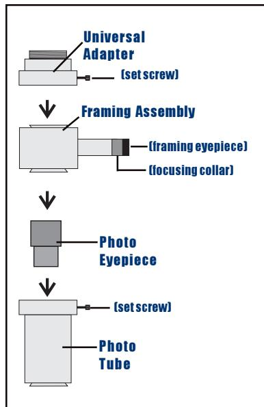
The diagram at left illustrates the basic configuration for photomicroscopy. Photography systems vary widely. Please refer to the assembly instructions, operating procedures and photography techniques for using specific cameras and photo systems, described in their respective instruction manuals. A valuable reference for Basic Photomicroscopy is:
