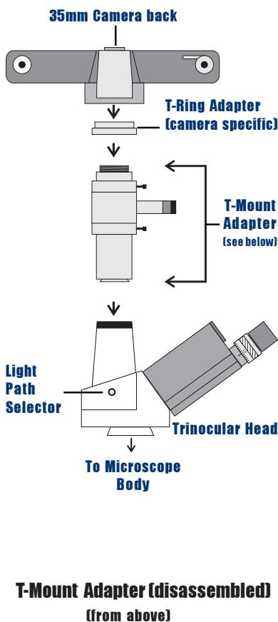
**T-Mount Adapter (disassembled)**
