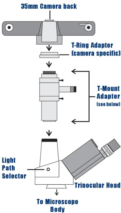
**T-Mount Adapter (disassembled)**
