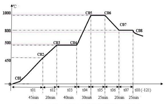
Figure I. Temperature Control Program with 8-segments
