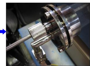
You may need "Pipe Twist" to tighten the Sealing Knob finally.
