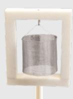
TGA-DTA sensor for hanging samples
