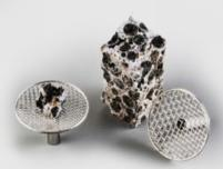
Pt/Ir net-shaped slip-on plates (ø 17 mm, 100/225 meshes/cm²)
