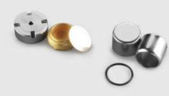
Medium-pressure crucible (right) and high-pressure crucible (left)
