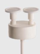
TGA-DTA sample carrier (with protected thermocouples) and slip-on plates for ASC operation
