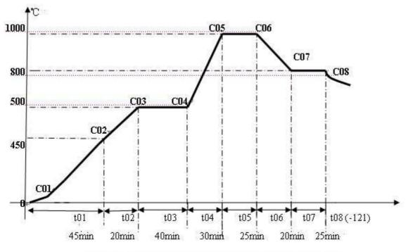
Figure I. Temperature Control Program with 8-segments
