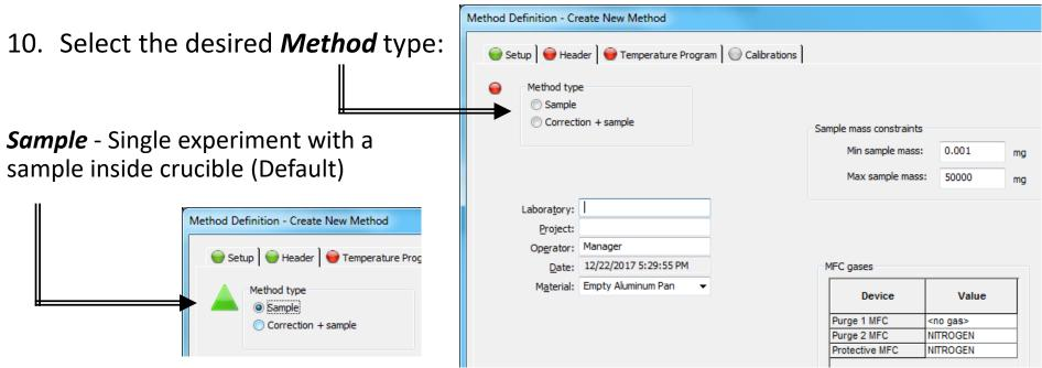
**Correction + sample** - Baseline correction experiments with empty crucible **BEFORE** single experiment with sample inside crucible – recommend if results are critical
